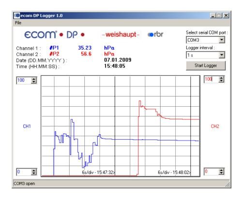
The measured value process of the ecom-DP can be logged with the help of the data logger program "ecom-DP Logger ". The program can be loaded free of charge from the download area of the rbr homepage www.rbr.de. To transfer the data a USB cable (kind becomes. - No.: 55818) and a driver (free download from www.seic.co.kr) is needed. The measured value rows can be stored in the xls format (Excel).
