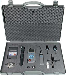
The final examination is performed with a visual check. In "normal" operation the usability test is done with the purpose of tracking down possible leakages. The gas loss in a pipe can be determined in litre per hour by the instrumentation.
